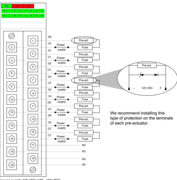
$\textbf{power supply} \ 125 \ VDC \ (100...150 \ VDC)$
