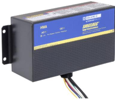
Surge protection device, Surgelogic, HWA, 100kA, 240/120 VAC HLD, 3 phase, 4 wire, NEMA 4X
