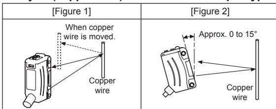
※Mount the sensor slanted at an angle ranged 0 to 15° shown above as [Figure 2] for stable detection to detect as shown in [Figure 1].
