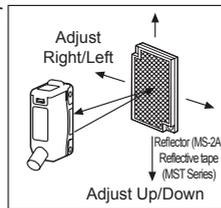
※Please use reflective tape (MST Series) for where a reflector is not installed.
