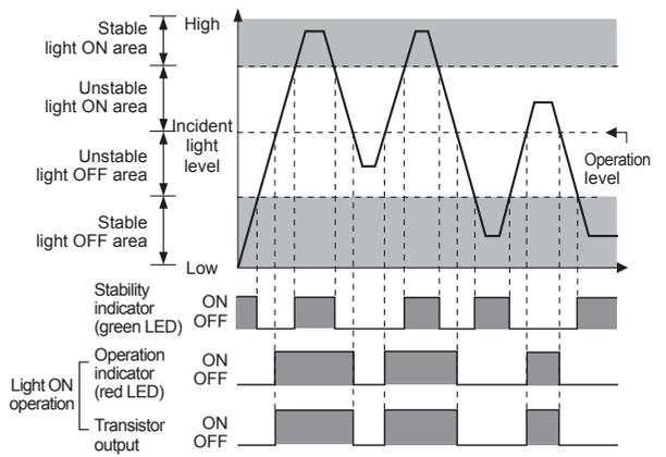
※The waveforms of "Operation indicator" and "Transistor output" are for Light ON operation.
